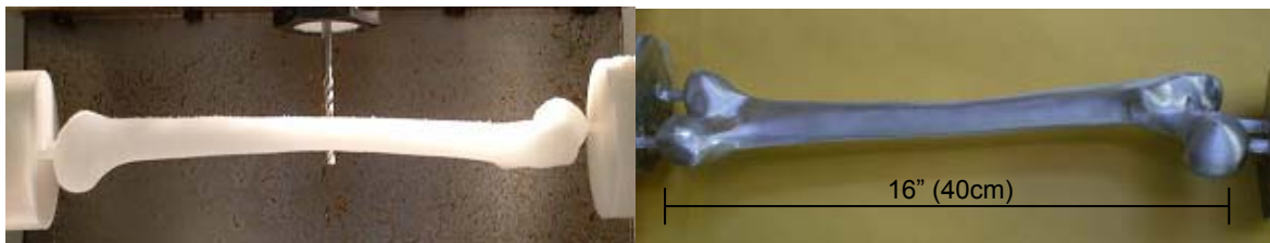
Figure 2 – Plastic (Delrin) and Aluminum human femurs created using CNC-RP
