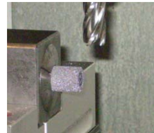
Figure 8 – TM sample fixtured in CNC mill
