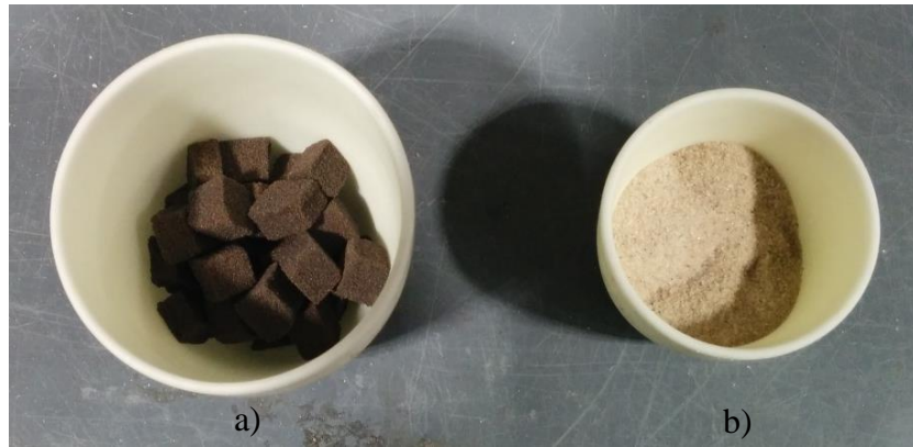
Figure 9. a) Printed ExOne Mold and b) Super Set 942 and TW30 after Binder Burnout at 450 °C
