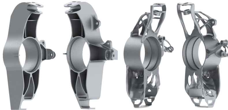
Figure 6: Redesign of an upright (left subtractive; right additive) Source: DMRC report 2012
