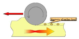
Fig. 11 Schematic view for compaction at high compaction factor
