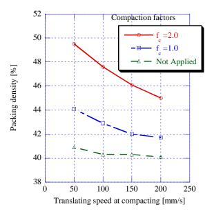
Fig. 6 Relationship between packing density and transverse speed
