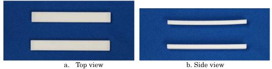
Fig. 9 Photos of specimens for curl distortion measurement. Top: without compacting, Bottom: with compacting.
