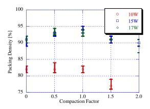
Fig. 8 Relationship between packing density of sinter and compaction factor
