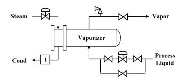
The minimum relief system design basis for a vaporizer that is normally open to the header is the vapor generation rate for blocked outlet.
