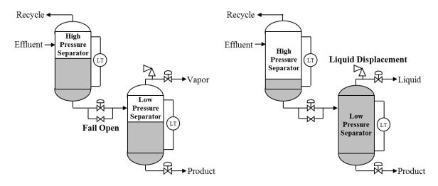
Besides simply preventing the low-pressure separator from becoming liquid full, the preference is to limit the maximum level to ensure the relief system is adequate based on 2-phase disengagement models and a check for liquid re-entrainment.
