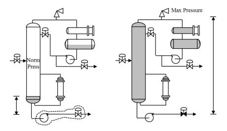
Figure 6: Overfilling of a Distillation Column
