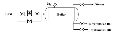
ASME Section  $I^{[6]}$  prescribes the relief system design requirements as the design steaming rate of the boiler. The underpinnings are that for BFW feed control valve fail open or inadvertent opening of the bypass, the boiler is open to the header.
