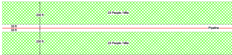
Figure 10. DOT Class 2 Population Distributions along the Example Natural Gas Transmission Pipeline (drawing not to scale)
