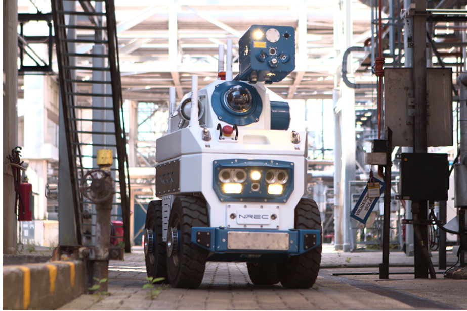
Figure 2.2: Sensabot Mark2 with boom mounted sensing payload for deployment in hard to reach areas. The cog rail system gears, for multi-level traversal, are mounted externally on the wheel hubs. [16]
