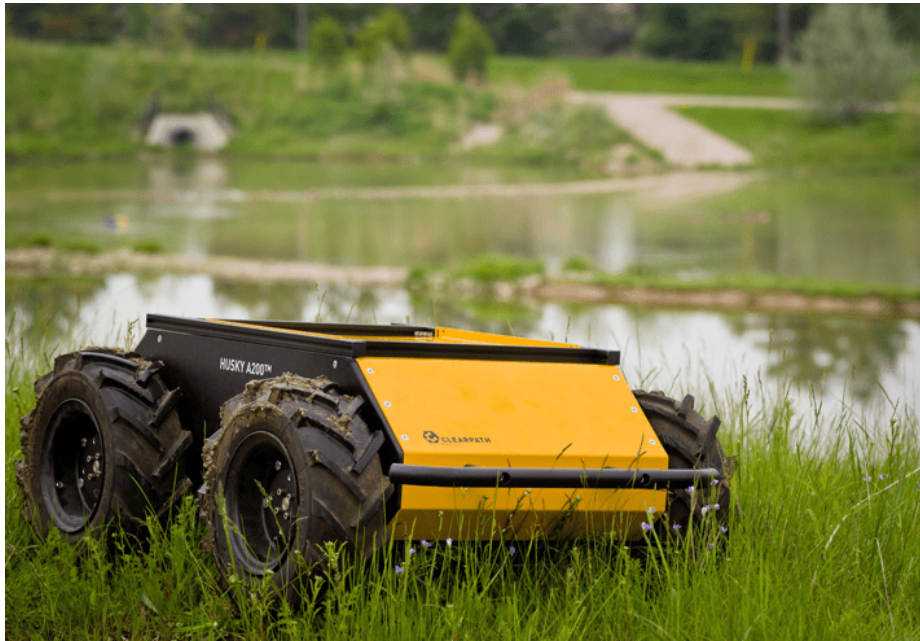
Figure 3.1: Clearpath Husky base without external sensor payloads. Large pneumatic tires allow the platform to safely travel across a broad spectrum of surfaces. [7]
