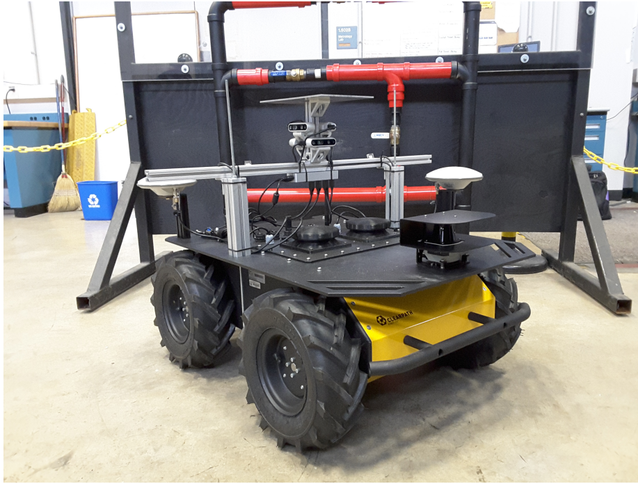
Figure 2.4: Differential drive autonomous ground vehicle robotic operator Philbart with LIDAR and GNSS receivers.
