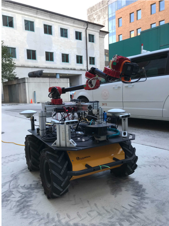
Figure 6.1: A HEBI manipulator with attached GoPro mounted on the Philbart mobile base.
