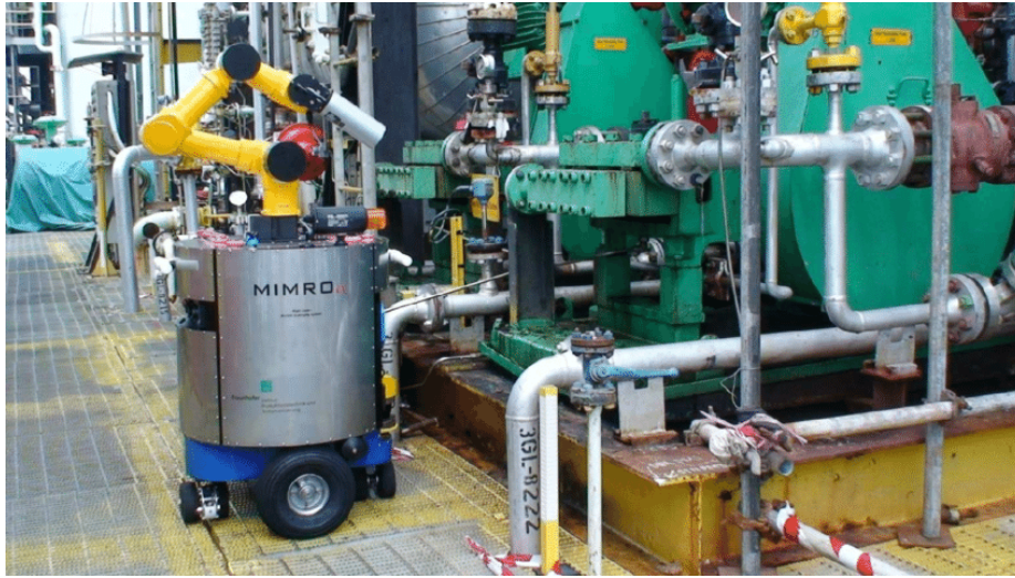
Figure 2.1: MIMROx deployed on an offshore production facility inspecting a component. [11]
