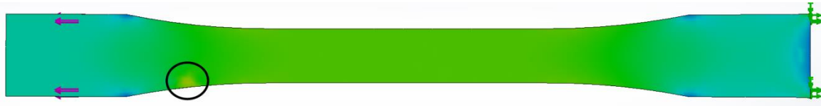
Figure 5. Von Mises Stress of a dogbone infected with a void.
