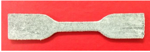
Figure 2 – ASTM Type IV Tensile Test sample (left) and dimensions (right) processed by HSS
