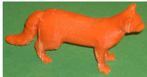
Figure 18: Cat part with the support structure removed [5]
