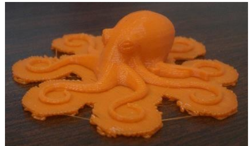
Figure 15: Octopus built with rafts to decrease warping
