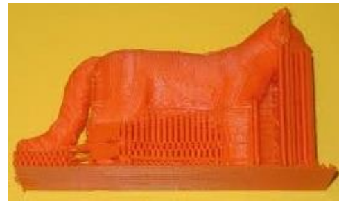
Figure 17: Cat part printed with supports in order to print its overhangs [5]
