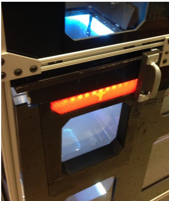
Figure 26: Vending bin open on the top to receive parts. In this position the drawer cannot open because it is blocked by the handle.
