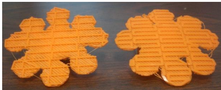
Figure 16: Standard raft on right and modified raft on left for easier part removal. The modified raft is less dense and has thinner lines.
