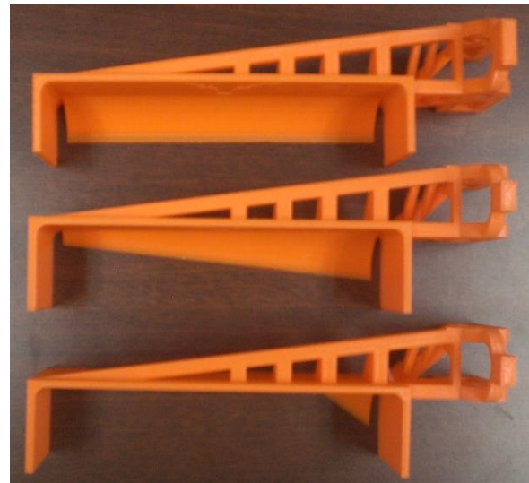
Figure 22: Sweepers with ramps for prying parts
