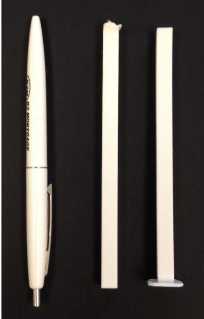
Figure 12: Tall part with small 7.5 mm square base, used for testing adhesion while building parts
