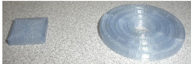
Figure 8: 15 mm square and 36 mm cylinder test parts
