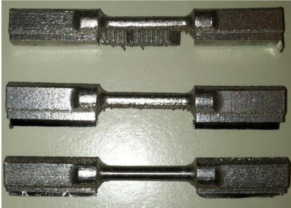
Figure 4. Tensile bar post-processing progression. Upper — block supports bonded to the reduced section, middle — support structures removed from the reduced section, lower — reduced section after light sanding on a lathe.
