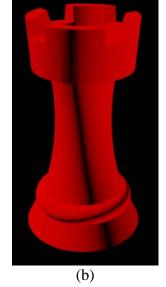
**Figure 1:** The AMF file can use a simple list of vertices and triangles to define a mesh and replicate the functionality of an STL file, but without leaks. The XML-compliant format makes storing, parsing, and reading the file easy.
