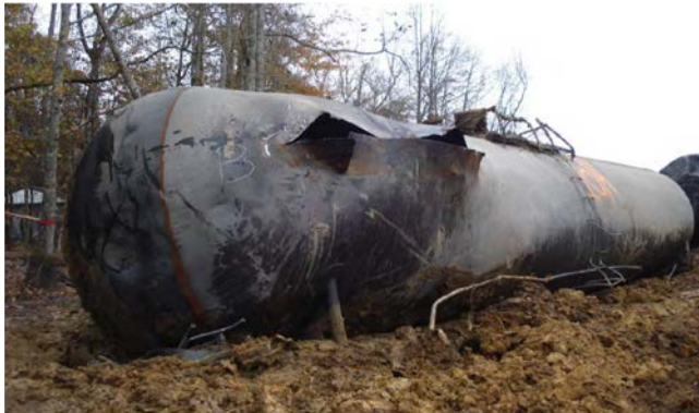
Fish-mouth tear in a tank car wall.
