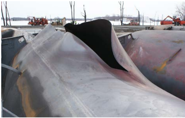
Fish-mouth tear in a tank car wall.
