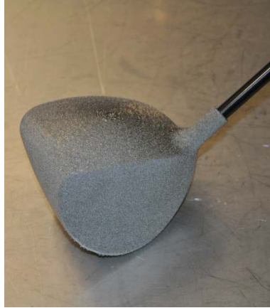
Figure 4: Titanium driver built using Arcam's EBM machine
