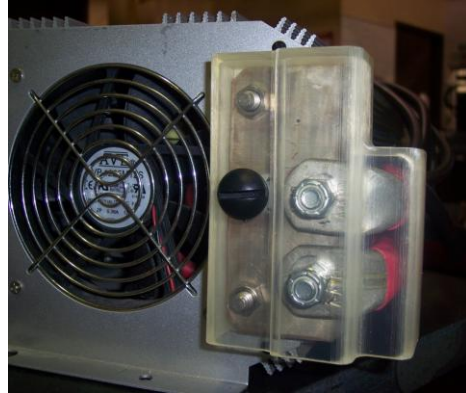
Figure 4. Battery terminal cap prototyping
