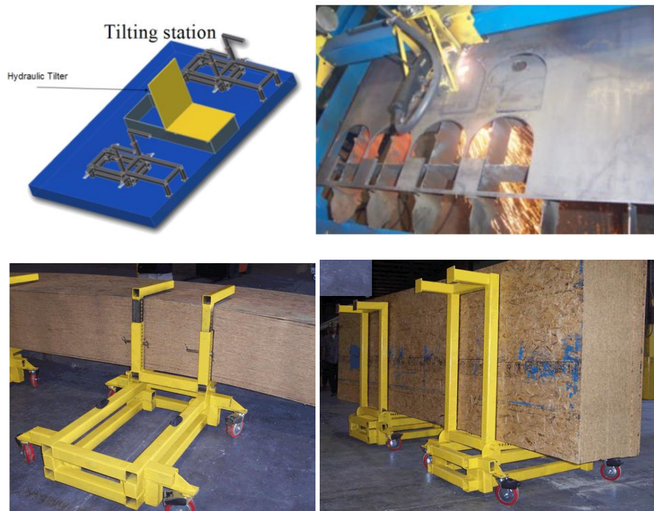
Figure 5. Tilt and transfer cart designing, manufacturing, and testing
