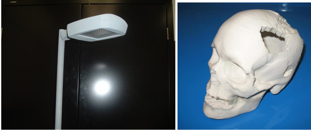
Figure 6. A light fixture prototype (left) and a rapid prototyped skull by the Zcorp 450 machine.
