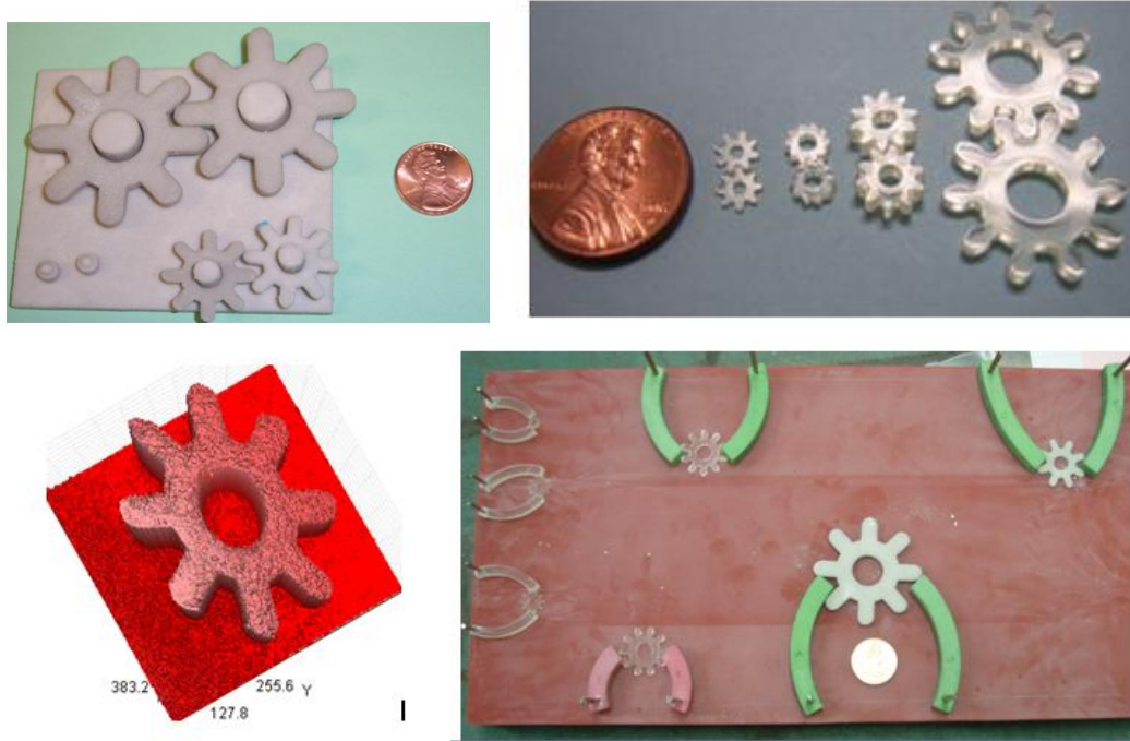
Figure 7. Rapid prototyping application in micro gear and gripper design and 3D Vision.
