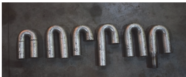
Figure 21 A part of tubular samples for geometric analysis of defined bending radius of 0.7D
