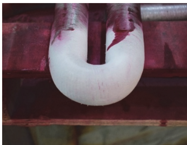
Figure 22 A capillary test
