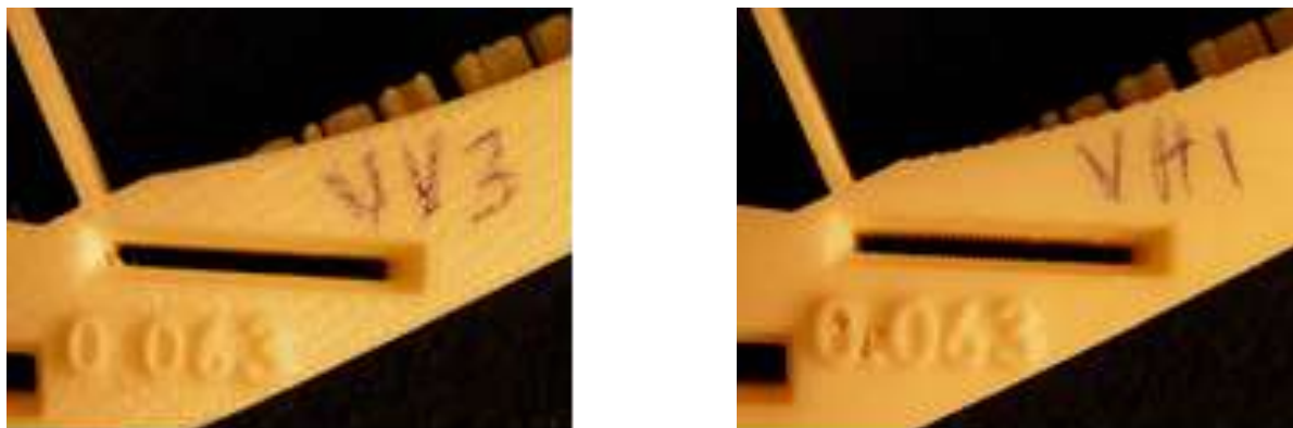
Figure 2. Photo record: Left is 1.6 mm slot printed vertically. Right is 1.6 mm slot printed horizontally; displaying more micro-scalloping in the horizontally printed slot.
