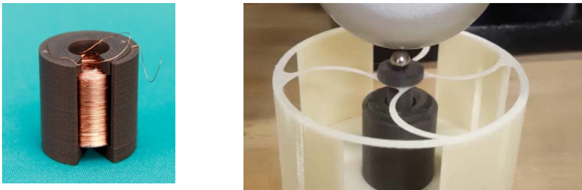
Fig. 9. (left) Multi-turn “thick” coil inside a cutaway iron-PLA frame; (right) electric bell incorporating coil, complete frame, ball-tipped moving plunger, and metal gong.
