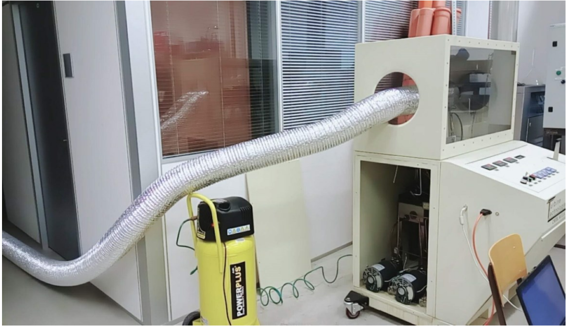
Figure 5.5 SR-30 Fuel Valve Operating System
