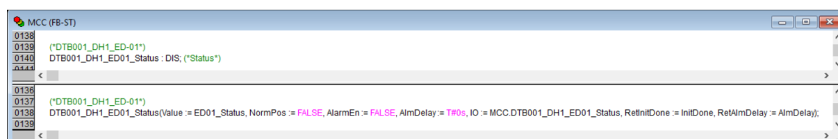
Figure 30 – Configuration of the status of one electric door
