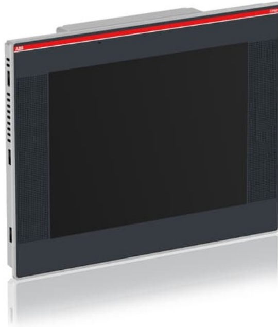
Figure 12 – The overview of the CP661-WEB panel [13]
