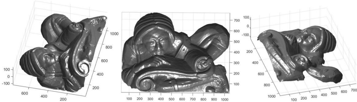
Figure 40 - Example of 3D reconstruction result using photometric stereo.
