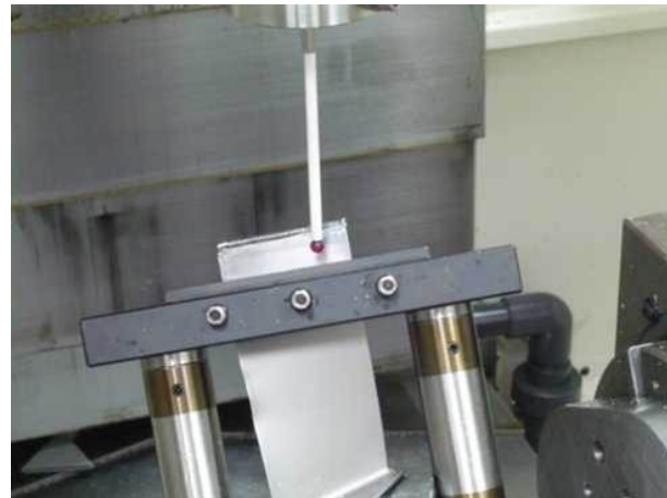
Figure 2 – Adaptively probing a compressor blade
