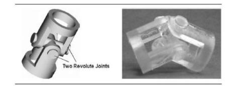
Figure 8: Universal joint built using SL [23]
