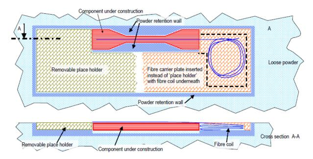
Figure 2: Top and side view of powder bed with component and fiber location [14]
