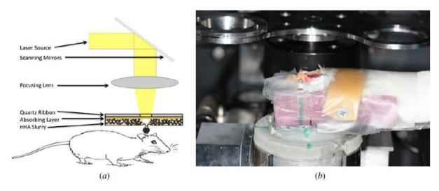
Figure 14: a) Schematic of setup for in vivo laser printing b) Specific holder for in vivo printing in mouse calvaria defects [28]
