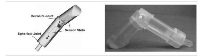
Figure 9: Robotic thumb built using SL [23]
