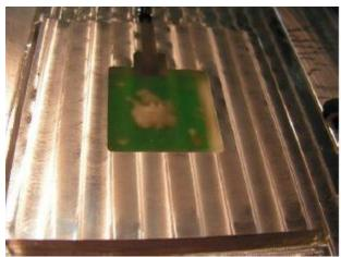
Figure 5: Sensor embedded using alumina filled potting epoxy [19]
