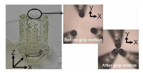
Figure 13: Fabrication and testing of three-grip micro-gripper [25]
