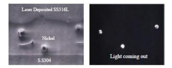
Figure 4: Embedded fiber optic sensors [16]
