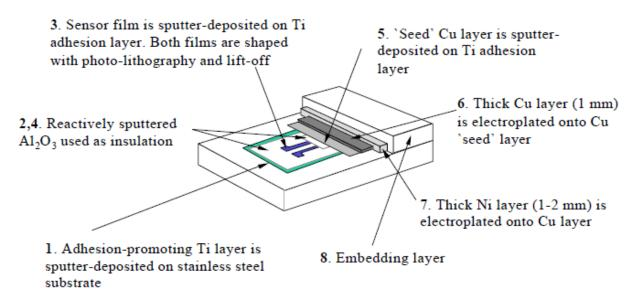
Figure 3: Procedure for embedding thermo-mechanical thin film sensors [16]
