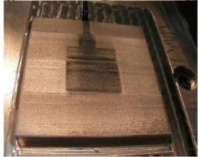
**Figure 6: Ultrasonic consolidation of aluminum onto embedded sensor** [19]
