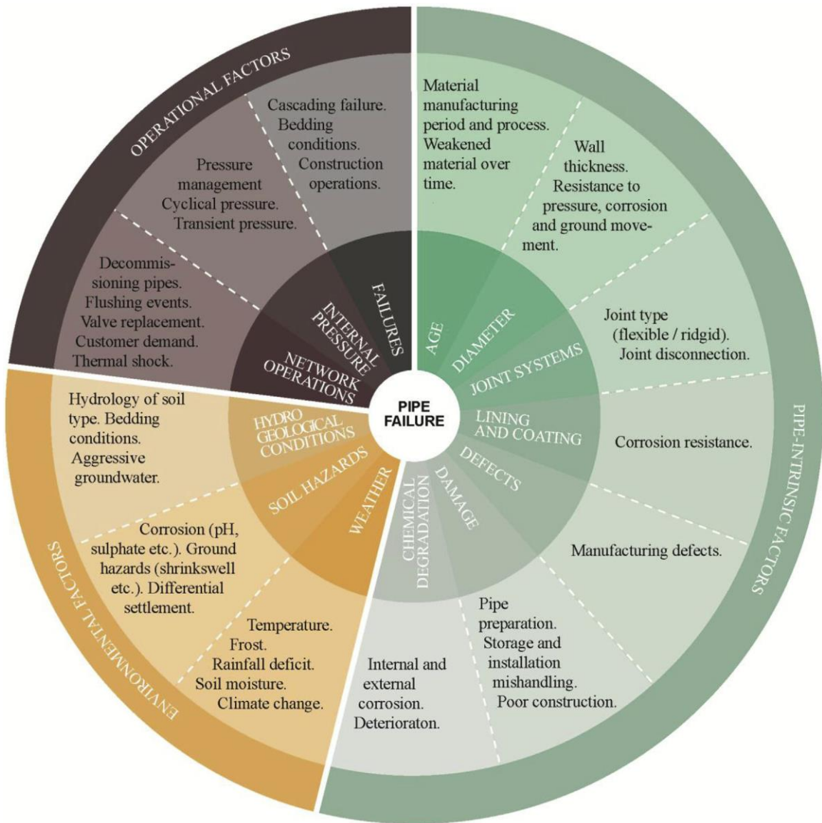
Figure 1. Categories of factors affecting pipe failure
