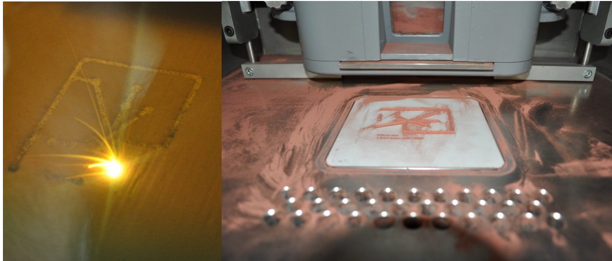
Figure 14 – Laser melting copper tracks in the SLM 125
