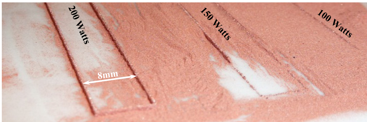
Figure 8 – Early conductive copper tracks on a decorative tile by SLM
