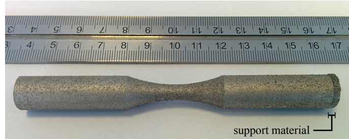
FIG. 2: SLM Al-Si10-Mg fatigue specimen. Note the additional 2 mm of supporting material at the specimen base, which was included to facilitate removal of the specimens from the SLM build platform.
