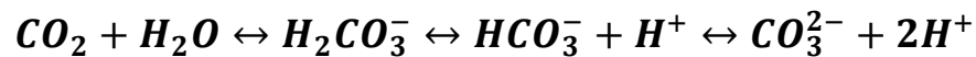
Figure 1: CO 2 dissolves in water to produce dissolved inorganic carbon (DIC) ions and hydrogen ions. An increase in hydrogen ions would lower the water pH.
