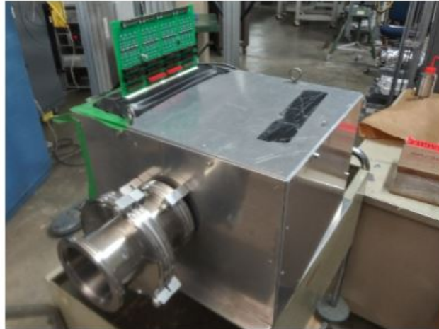
Figure 2.6: Detector assembly and electronics within the closed aluminum box
