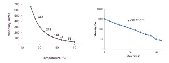
Figure 4 (a) Viscosities under different temperature, ink 3. (b) Viscosity under different shear rate, ink 5, 25°C
