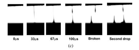
Figure 7 Jetting process of (a) low viscosity, (b) medium and (c) high viscosity inks
