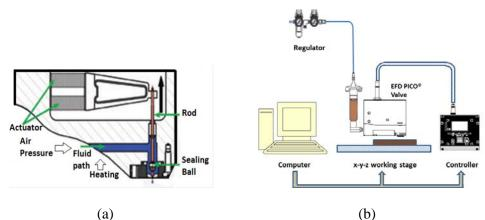
Figure 1 Schematic of the PicoDot<sup>TM</sup> jetting valve (a) and the 3D jetting system (b)
