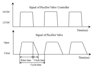
Figure 3 Signals generated by the jet valve controller
