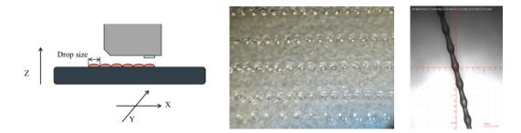
Figure 8 (a) Pattering process, (b) droplets pattern and (c) jetted fiber of pseudoplastic fluidic
