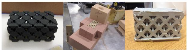
Figure 2. a) Complex printed mold created using binder jetting, b) no-bake outer mold, and c) cast complex structure
