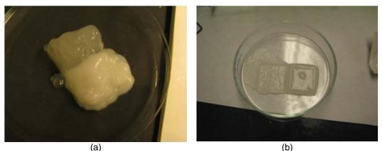
**Figure 5: CAD Model and Corresponding Hydrogel Prints**. (a) A manual print was made first to test the effectiveness of the method. (b) This proved successful and thus, a Fab@Home print was also made (1" by 2" by ~0.04").
