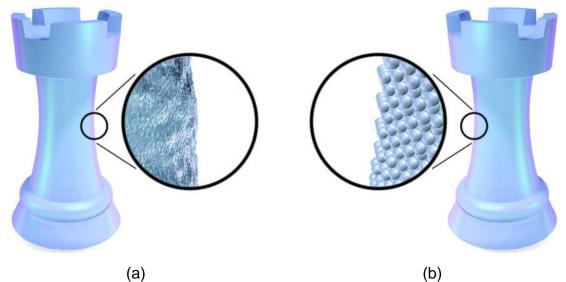
**Figure 1:** Traditional analog materials (a) are continuous in nature and every dimension has an associated finite error. Digital (discrete) materials are composed of fundamental, aligned building units (voxels) and the structure is defined perfectly by the presence or absence of a voxel at each location within the lattice.
