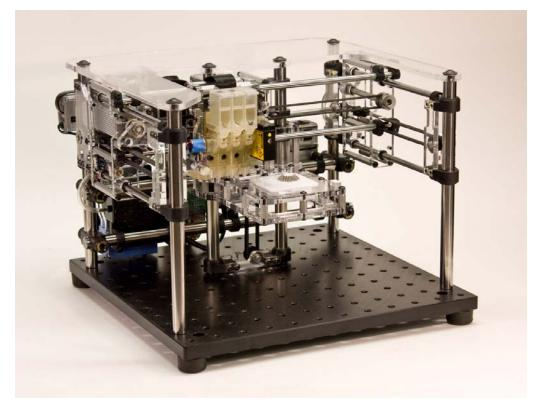
**Figure 2:** The VoxJet research platform was used to quickly and autonomously build multi-material structures made of hundreds of 1.5mm spherical voxels. The system also deposits binder to hold the structure together and includes error correction via closed loop deposition feedback.
