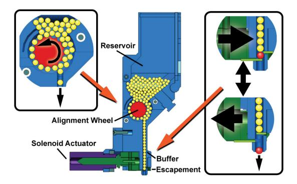
**Figure 3:** A cutaway diagram of the material deposition modules. Loose spheres are poured into the reservoir, which are aligned into a one-dimensional buffer by the continuously rotating alignment wheel. A solenoid actuated escapement mechanism deposits precisely one sphere with each cycle, and can reliable deposit up to ten spheres per second.
