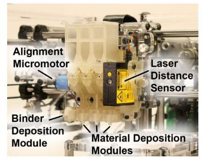
**Figure 4:** The deposition head consists of a binder depositing system, three separate material deposition modules, and a laser distance sensor. As the print head scans from right to left, binder is deposited appropriately, followed by spheres of any available material. The laser sensor verifies the placement of each sphere.
