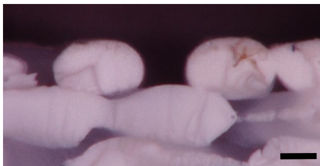
Figure 3. Cross section of FDM microchannel, perpendicular to the length of the channel. Scale bar: 200 \mu\text{m} .
