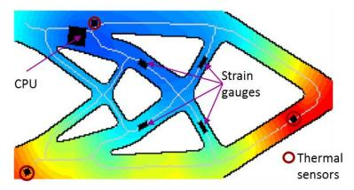
Figure 5: An example demonstrating component placement based on performance measures.
