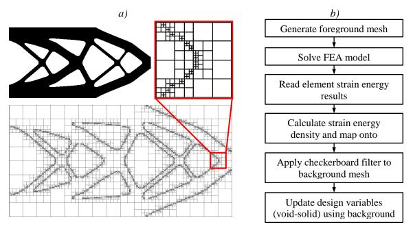
*Figure 8: a) An octree decomposed topology used for analysis, b) Integration of meshing procedure into BESO TO routine.*
