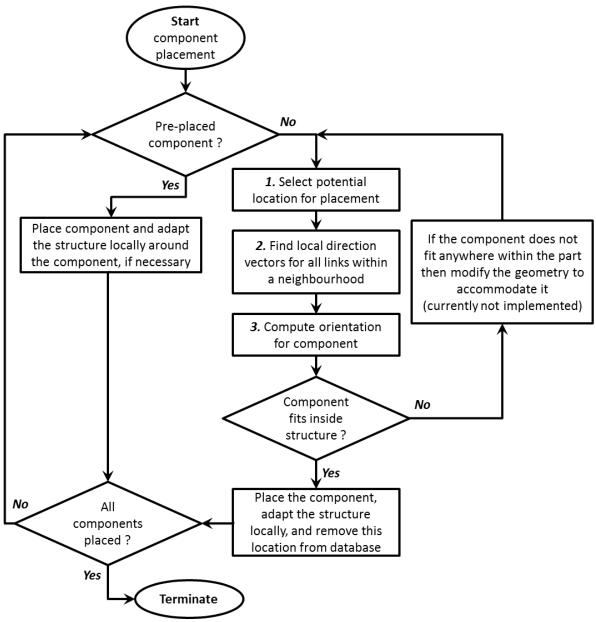
*Figure 6: The placement methodology*
