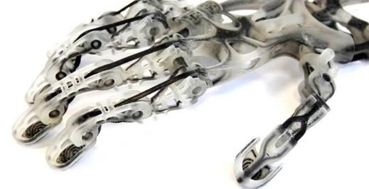
Figure 1: Multi-material jetted concept prototype - a) an example of a topologically optimized structural part with integrated internal system of placed components and the associated routing, b) a prosthetic arm with embedded systems and the associated routing [2], and c) a zoomed-in view of the prosthetic arm highlighting the complexity of the hand.
