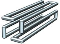
Figure 10 – Example of design freedom in creating a compact 3D strain gauge to be placed in thin structural members.
