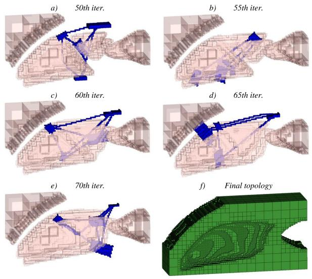
Figure 9: Results for test case 1 – coupled optimization strategy Internally placed components and associated routing shown for a) 50th iter b) 55th iter c) 60th iter d) 65th iter e) 70th iter f) final topology
