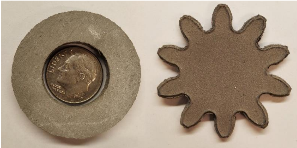
Figure 9. SSS printed 316L stainless steel parts
