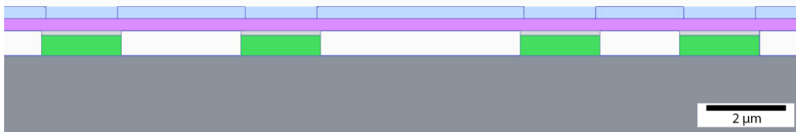
Figure 3.9: Scale drawing of a sample that has been transferred onto a partially supported measurement device. All EBL steps have been performed and the assembly is ready for metal deposition. The supported device consists of the silicon substrate (gray), nitride beams (green) and contact metal (silver). The sample and oxide beam (purple) have been transferred onto the device using a PMMA carrier layer (blue), which has been patterned using EBL. The sample is attached to the bottom of the oxide beam and is not in direct contact with any polymer layers.
