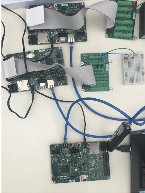
Figure 11: Recovery Igniter System Test Flight Computer Setup.
