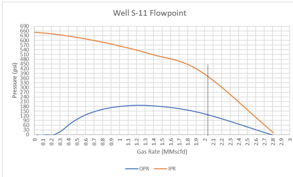
Figure 70 - Well S-11 flow-point analysis plot
