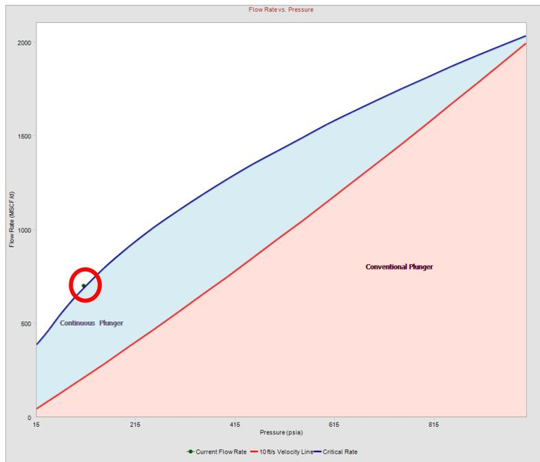
Figure 46 - Well S-5 PAGL plot with 2-7/8" tubing
