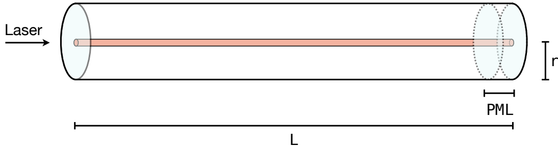
Figure B.2: Illustration of the PML region in the fiber amplifier model. A small layer with complex coordinate stretching at the fiber end is sufficient to absorb the outgoing wave.
