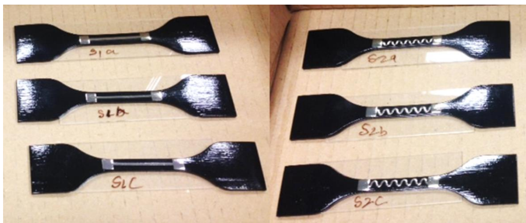
Figure 5 A photographic image showing the inkjet printed silver tracks (straight line and sinewave track patterns) on the tensile bar specimens
