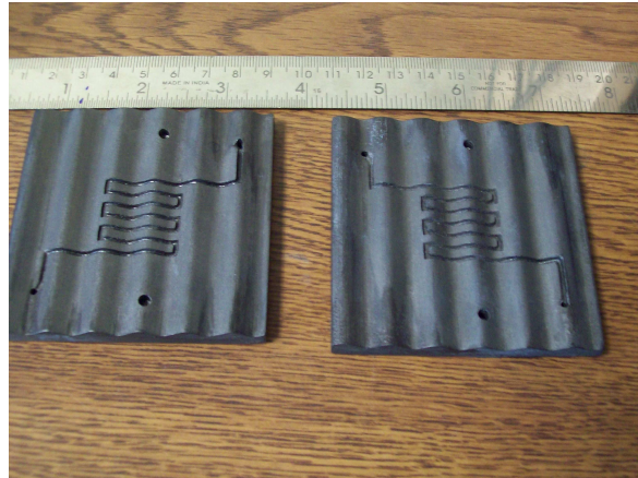
Figure 1: Corrugated plates with 10% more surface area compared to a flat plate. The channel dimensions are 2 mm.
