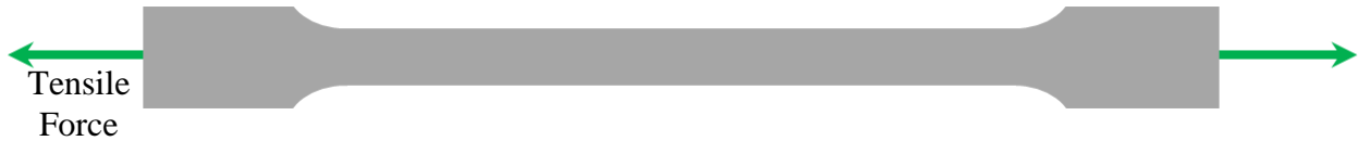
Figure 6: Tensile test schematic (shown horizontally).
