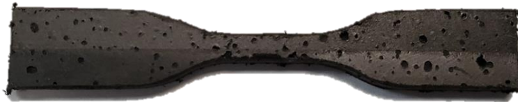
Figure 3.21 ASTM D638 type V tensile bar machined from RF-sintered specimens
