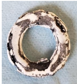
Figure 6.3 Fused ring geometry after two-stage heating where the powder bed was heated for one minute in each electrode configuration. Top/Bottom and Left/Right refer to the position of the electrodes with respect to the image.
