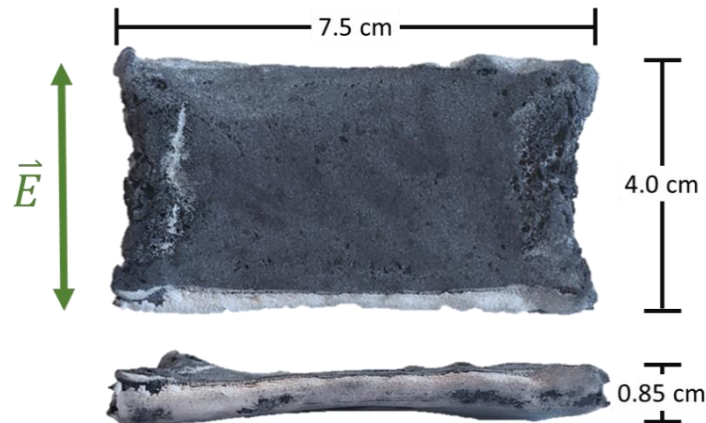
Figure 3.19 Fused part created from a selectively doped powder bed in which the geometry was defined by a rectangular cross section. The doped region contained 30% graphite by weight, and the part was exposed to RF radiation for six minutes.
