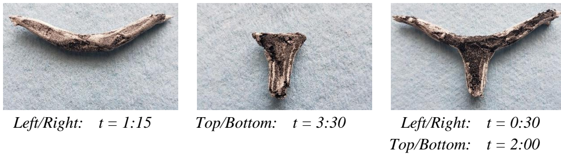
Figure 6.4 Fused parts from uniform dopant concentration after heating in multiple electrode configurations with corresponding RF exposure times in minutes. Top/Bottom and Left/Right refer to the position of the electrodes with respect to the image.
