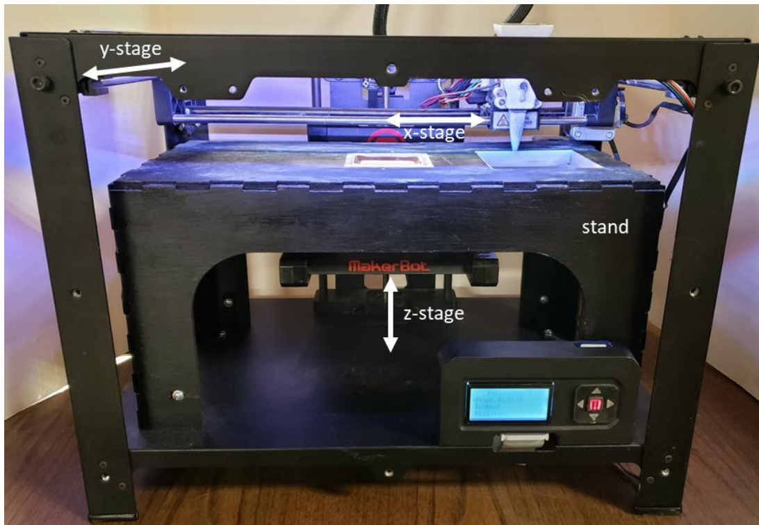
Figure 5.1 MakerBot Replicator 2 modified to pattern doped dry powders. The 3 axes of movement and their respective stages are labeled.
