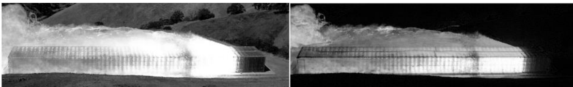
Figure 22. Original grayscale image (left) and the same image with reference pixel intensities subtracted (right)
