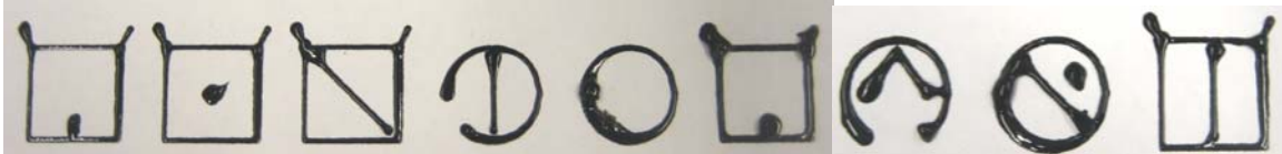
Figure 13. Printing WindowArt with Red Tip: WindowArt is printed with considerable precision using the red flexible tip.
