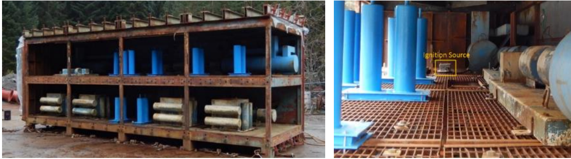
Figure 2: 50 m 3 test rig in the congested configuration.
