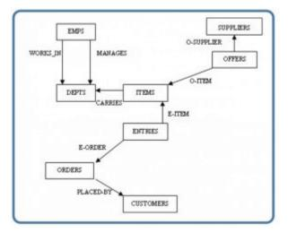
Figure 4.1. Network model diagram.
