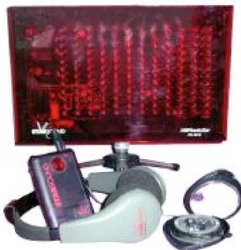
Figure 5. Infrared hearing enhancement system by Phonic Ear (Centrum Sound Systems, 2007)
