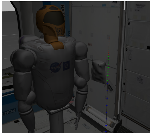
Figure 2.15: Simulating collaboration with ROS enabled platforms to complete tasks aboard the International Space Station.
