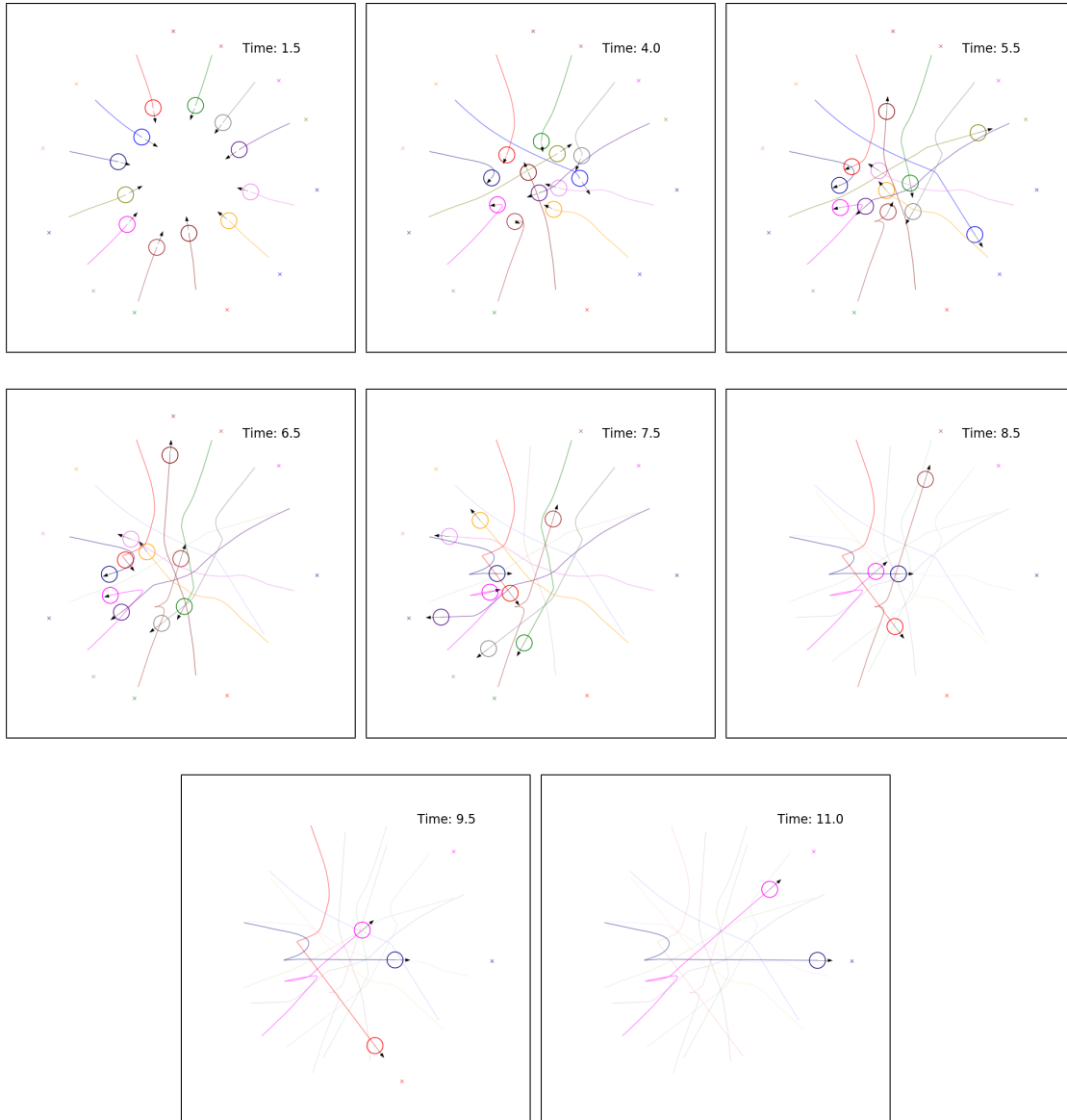
Figure 4.4: Vanilla ORCA simulation on 12 agents Circle scenario with agent-radius set to 0.25m. The last three agents exhibit high rotation and end up travelling a longer and convoluted distances to the goal with extreme curvatures.
